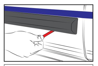
**STEP 5:** Ensure Body Side Molding is positioned correctly on the door surface before applying light pressure to the exposed tape areas. Slowly peel the remaining tape liner away by pulling on the exposed ends of liner and apply firm pressure around the attachment areas.
