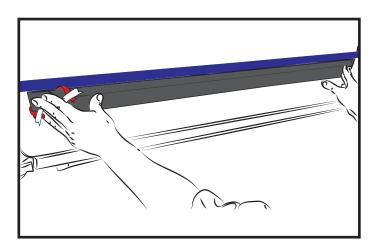
**STEP 4:** Aligning the rear end of Body Side Moldings with the position noted in step 2. Position the Body Side Molding so the top edge of part is running parrel along the base of the ridge line profile in the door surface. Ensure the tape liner along top, bottom and ends are on the ouside edge of Body Side Moldings.
