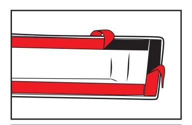
**STEP 3:** Peel back approximately 2" inches of protective tape liner and fold to the outside of Body Side Moldings at a 45 degree angle along top, bottom and ends of Body Side Moldings. **Important: Do not touch the exposed surface of the tape.**
