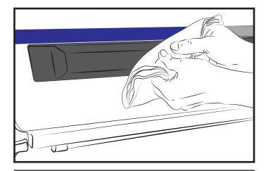
**STEP 6:** Using a clean, soft cloth, firmly rub down over the attachment areas to ensure maximum adhesion. Ensure top, bottom and ends of Body Side Moldings are rubbed down 5 times using firm pressure along tape attachment areas. Ensure no gapping is evident along top, bottom and ends of Body Side Moldings.
