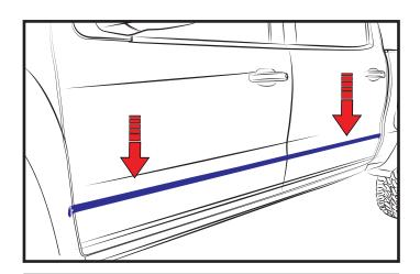
**STEP 1:** Clean the door areas where the Body Side Moldings will make contact with the door surface. Ensure doors are dry prior to install. Apply masking tape to front and rear doors along the top of the ridge line in the door profile. Ensure the masking tape is in a straight line to assist with aligning the Body Side Moldings to the front and rear doors.
