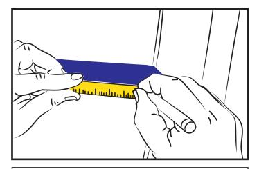
**STEP 2:** Using a ruler measure in 2 cm inch from the back end of front and rear doors marking the position with a non-permanent marker on masking tape. Ensure the correct Body Side Moldings are identified prior to installing to front and rear doors. Parts are identified on the back side of Body Side Moldings.
