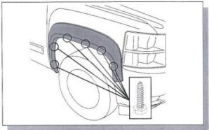
8. Re-Install the socket head screws into the fender to secure the Fender Flares. Fit the Fender Flares loosely until the Fender Flares are aligned as desired, when satisfied, tighten the screws fully and ensure extrusion is flush neatly against the body.
