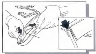
Pulling at right angles to the extrusion, remove the liner from the extrusion in small portions and apply thumb
