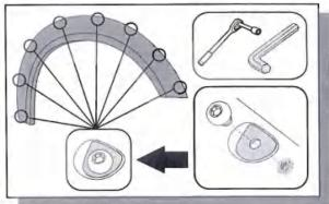
Attach bolts to each Fender Flare using a 3/16" Allen key and a 1/2" wrench/socket.
