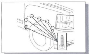
6. Use the original manufacturer's hardware that is in the wheel arch of the vehicle to fit the Fender Flares. Remove the 6x 7mm socket head screws from the fasteners on the vehicle.
