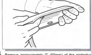
3. Remove approximately 2" (50mm) of the protective liner from the extrusion. Fit the extrusion to the Fender Flare along the edge that comes in contact with the vehicle's body panel.
