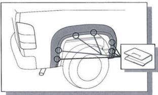
7. To secure the Fender Flare to the body, take the black metal clips and slide them over the Fender Flare and inner wheel arch lip. Position clip so that the barb in the clip locates in the slot in the Fender Flare. Ensure all fixing points are secure and that extrusion is flush neatly against the body.
