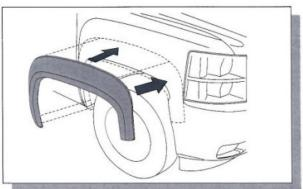
Place the Fender Flares onto the vehicle and line up the holes on the part with the screw holes on the vehicle.
