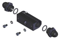
21. Thread the o-ring side of each P/N 15607 port fitting into the back ports of each fuel rail.
