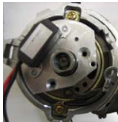
Figure 2 Install module on top of adapter plate and secure both plates with provided screws.
