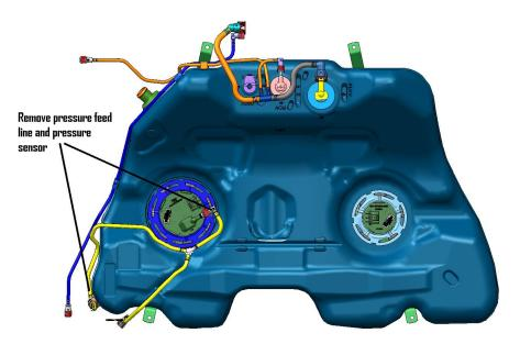
12. Carefully remove the fuel pump assembly as not to bend the float arm. There will also be a fuel transfer tube located on the bottom side of the assembly. Release this connection and let it fall back into the tank. The figure below gives you a visual on the internal working of your fuel tank. **FIGURE 1-3**
