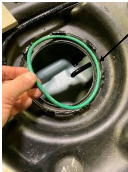
Install new fuel pump module gasket (not included). Use Dorman PN: 911245 or equivalent.
