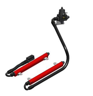
27. Assemble a hose with a straight AN-08 hose end on one end with a 180 degree hose end on the other. Attach this hose to the front of the passenger side rail using the 180 degree end. Place the pressure sensor re-locator on the other end as pictured.
