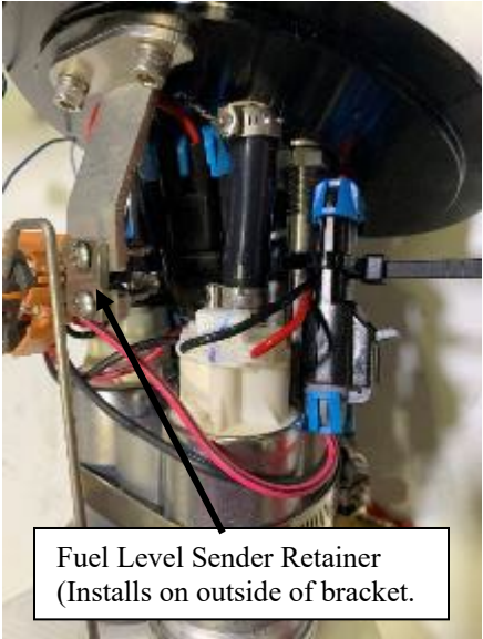
Install fuel level sender retainer and secure with 6-32 screws, washers, and nuts.
