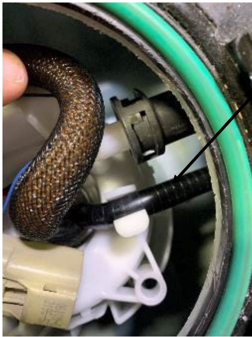
Internal Siphon Return Line – Remove from plastic clip.
