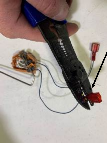
Crimp male spade connectors on fuel level sender wires.
