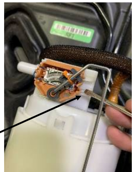
Depress small plastic tab to release fuel level sender from lower fuel pump module mount.
