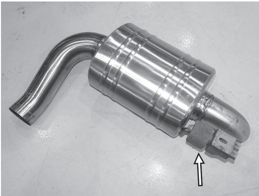
9) Install the factory exhaust hanger assembly onto the APR rear muffler in the same orientation.
