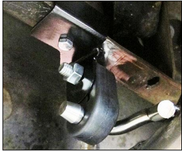
Figure 4 – Right tailpipe hanger bracket
