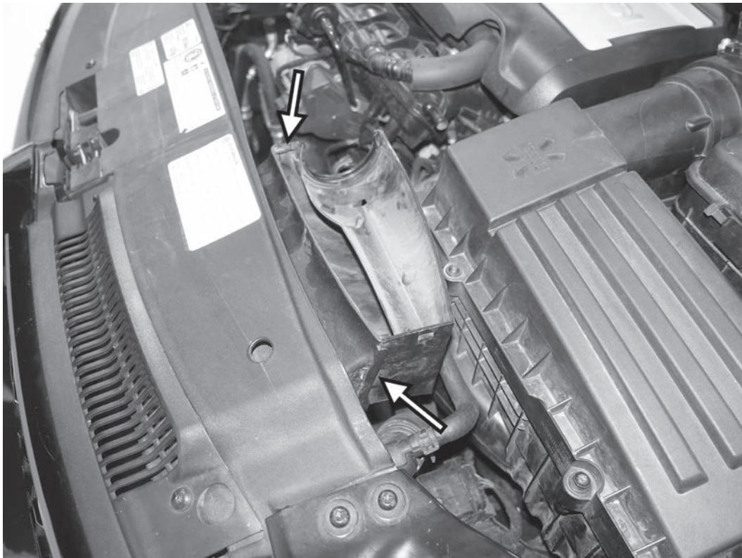
3) Press in the tabs on both sides of the inlet scoop, and rock the inlet scoop back to separate the inlet scoop from the radiator core support. Remove the inlet scoop from the car.
