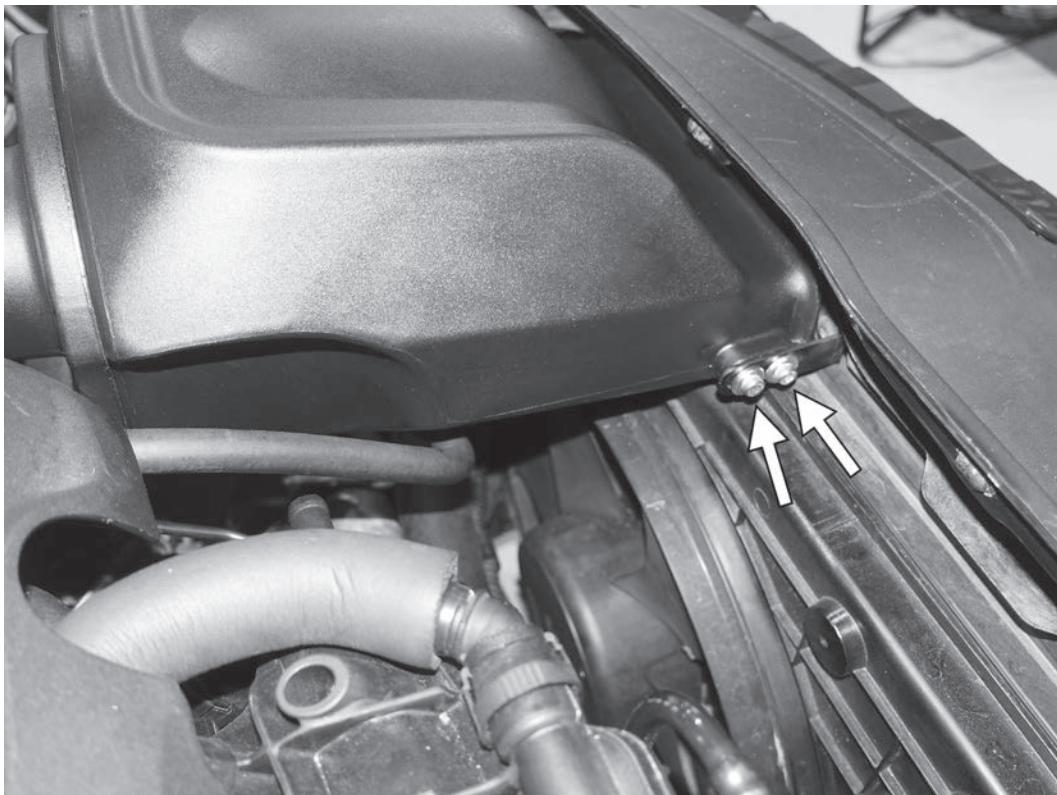
15) Using the supplied blue thread locker on the screws, install and tighten the two 3mm allen screws with washers to hold the front "L" bracket to the mounting boses on the front right of the APR intake.
