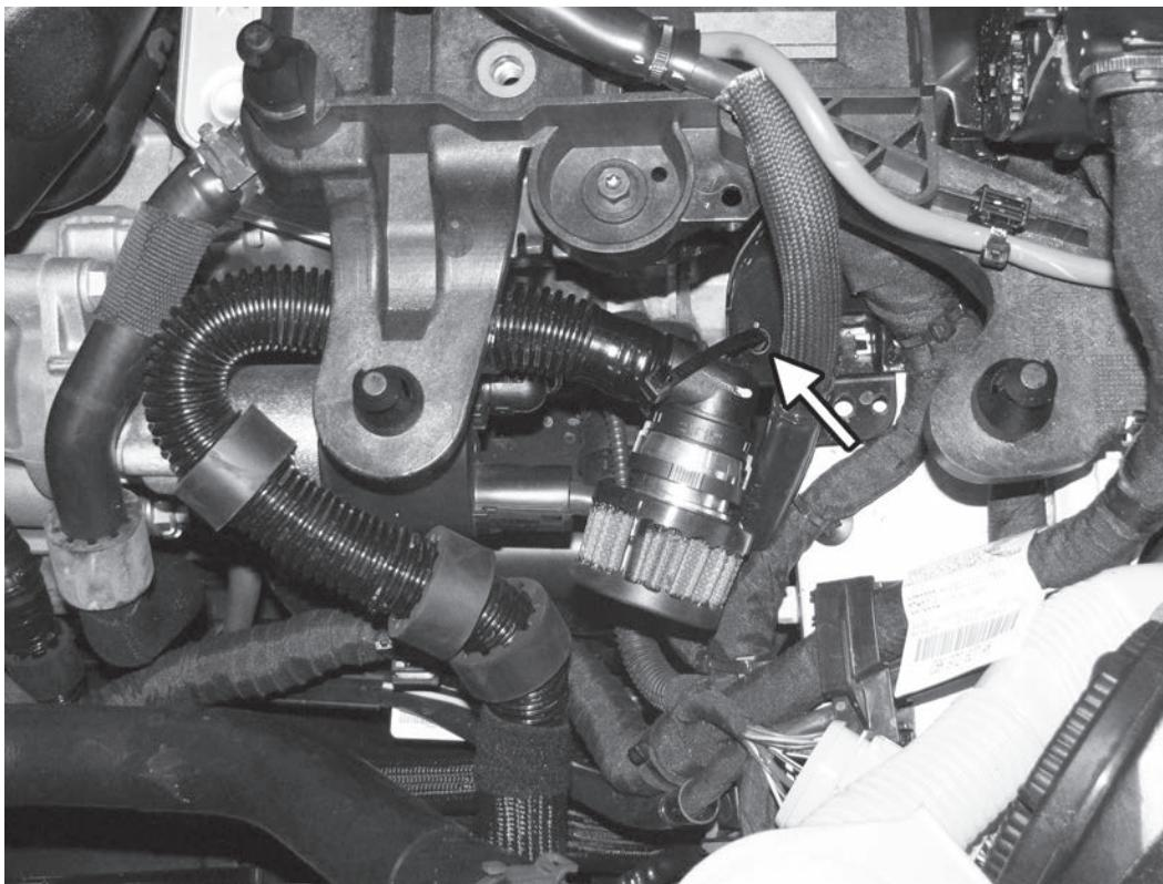
17) If equipped with Secondary Air Injection, clip the APR secondary air filter (Sold separately as CI100020-A) into the factory fitting on the end of the secondary air pipe. Bend the pipe to tuck it out of the way and secure it with the supplied cable ties.
