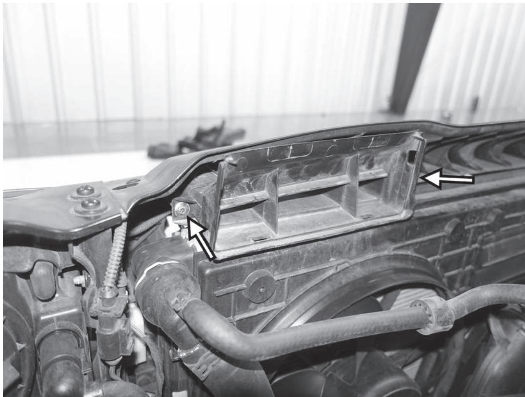
9) Unscrew the two T25 screws holding the front of the airbox inlet scoop from the back of the radiator core support.
