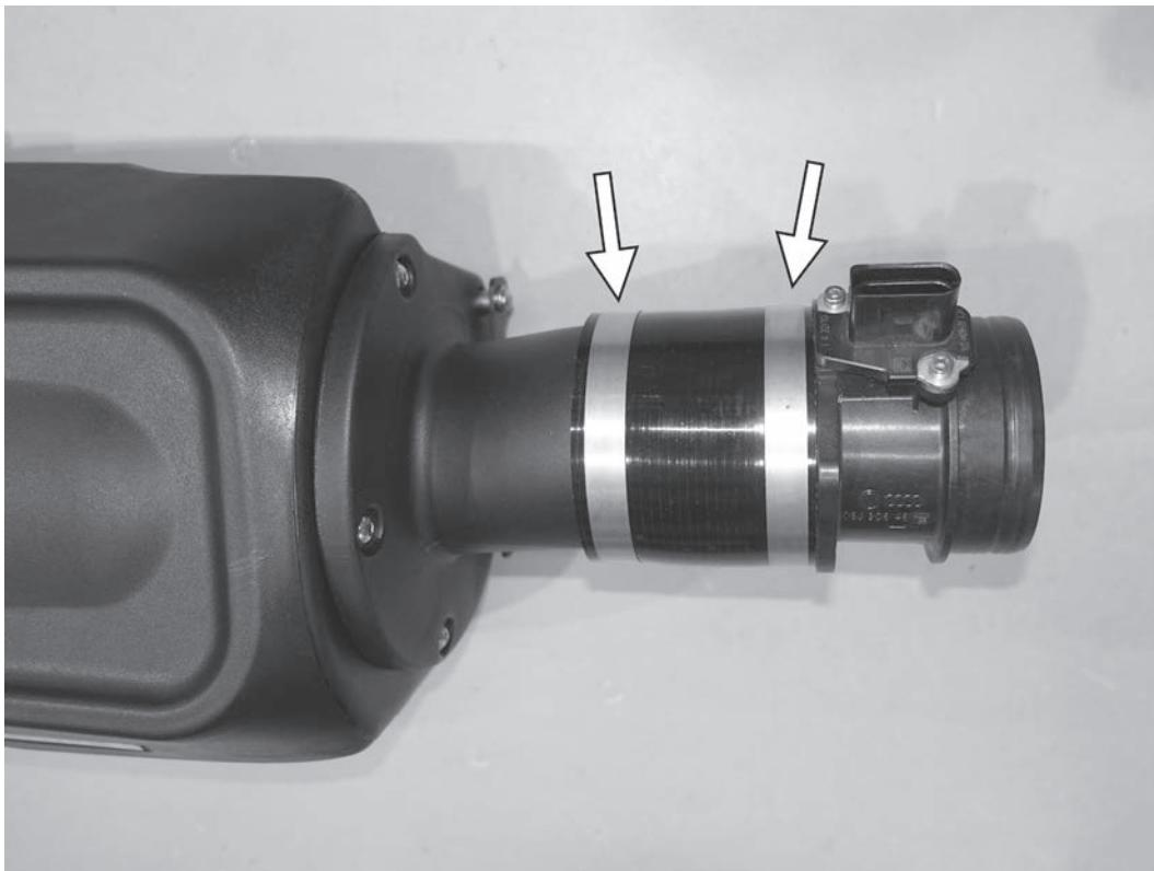
11) Using the supplied silicone coupler and two hose clamps, loosely install the MAF sensor to the back of the APR airbox in the same orientation as the with the stock sensor.
