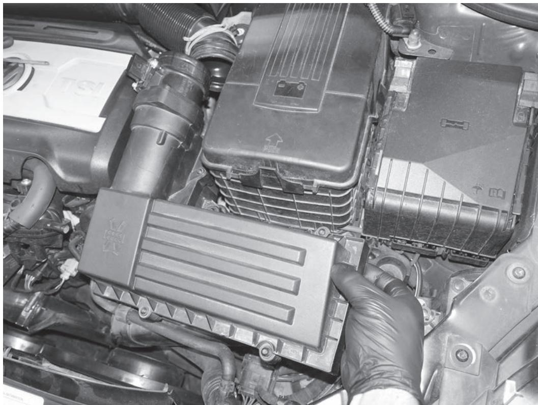
7) Lift the left side of the airbox up to pull off the rubber mounting post underneath. Lift the right side of the airbox from the other rubber mounting post to separate the airbox from the car.
