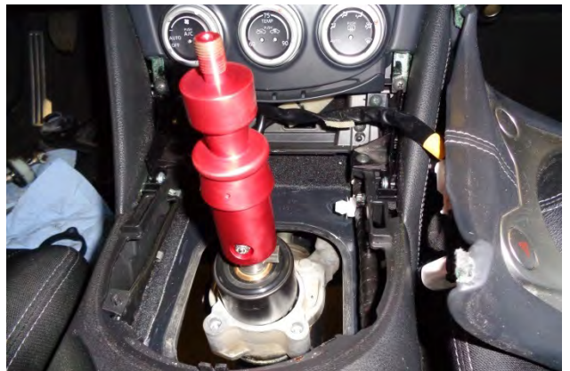
22. Place shift lever assembly (5) on top of the spring.
