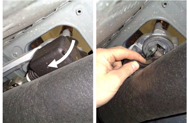
15. Underneath the vehicle, expose the shift link bolt by pulling the lower dust boot off of the shifter housing and pushing it forward.
