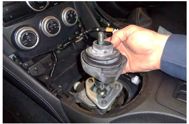
14. Pull the inner dust boot off of the shifter plate and lift it over the shift lever.
