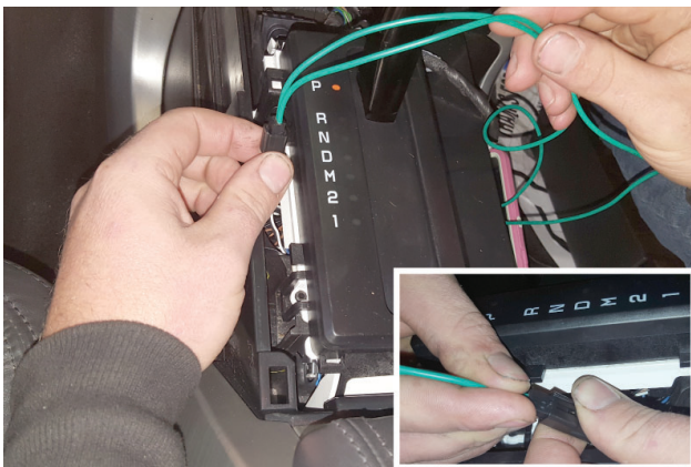
14. Route switch assembly wiring over to tow/haul button wires (from step 7), connect them and tuck wiring down out of the way.
