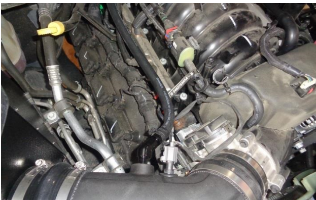
33. Apply 2 wraps of nylon thread tape to the 1/2" straight barb fitting (18) and install it in the 45° elbow (17). Apply 2 wraps of thread tape to the elbow and install it in the intake tube, aligning it as shown. Cut the 1/2" hose so that it lays as shown, then use the pinch clamp (19) to secure it to the fitting.
