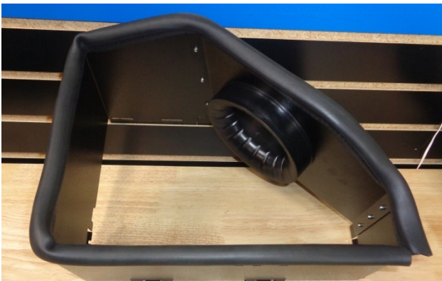
14. Attach the gasket (5) to the heat shield. Firmly press the gasket onto the edge, gradually working around the heat shield. When you return to the starting point, trim the gasket to fit using metal-cutting shears.
