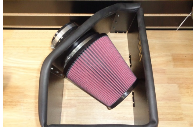
16. Place the clamp (2) on the air filter (1), install the filter on the filter adapter and tighten the clamp.
