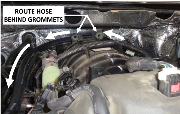
32. Route the 1/2" hose behind the two engine cover mount grommets, then forward toward the intake duct.
