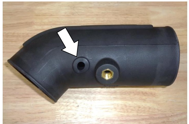
18. Insert the rubber grommet (14) into the intake tube (16). NOTE: Moistening the grommet with soapy water will ease insertion.
