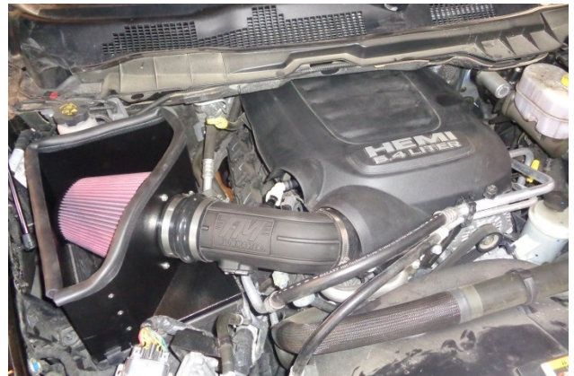
34. Reinstall the engine appearance cover by pushing the two rear pins into their grommets, then pressing the front down onto the two friction pins.
