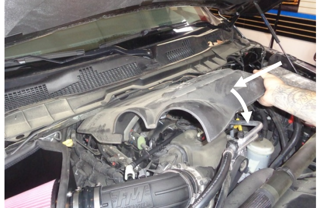
34. Reinstall the engine appearance cover by pushing the two rear pins into their grommets, then pressing the front down onto the two friction pins.
