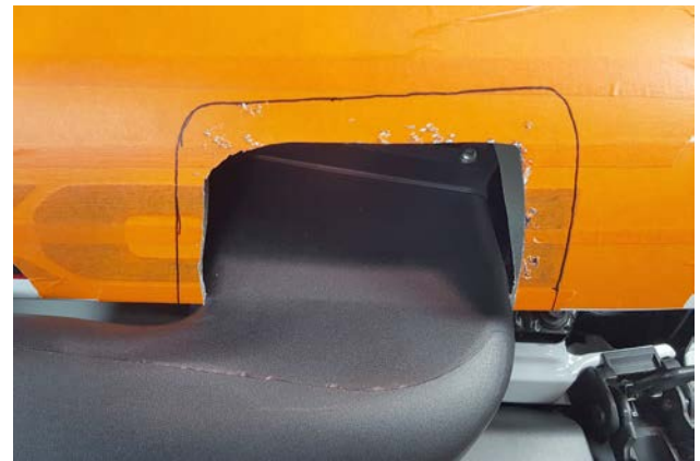
44. Make a cut well within marks through both layers of hood, then lower your hood so you can inspect location of cutout. That way you can adjust it front or rearward so it fits better.
