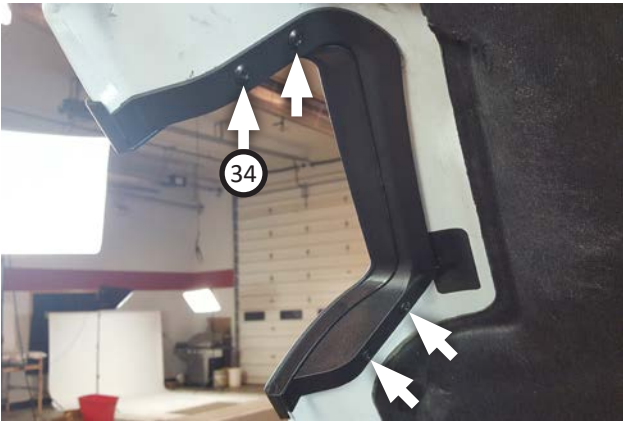
59. Fasten inner hood gasket to hood using (x4) blind rivets (34) through holes drilled in previous step.
