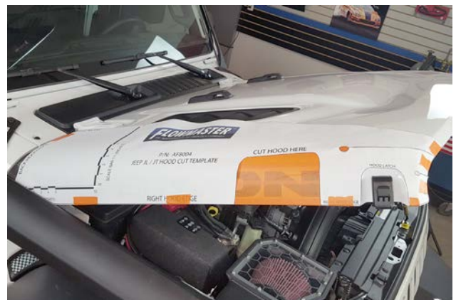
41. Fold template back onto hood and after re-aligning it, tape it down. Tape front portion down one piece at a time as shown.
