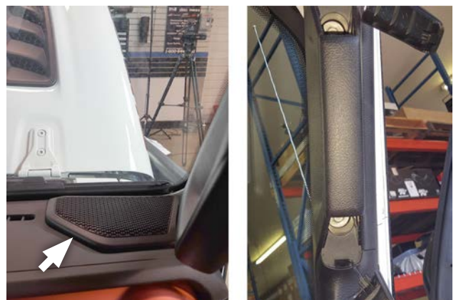
23. Release cover from base of A pillar then remove bolt covers from passenger grab handle on A pillar.
