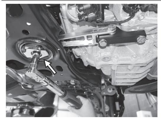
5) If using an APR bolt, torque the rear bolt to 100Nm (74 ft-lb).
