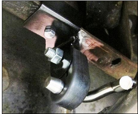
Figure 4 – Right tailpipe hanger bracket
