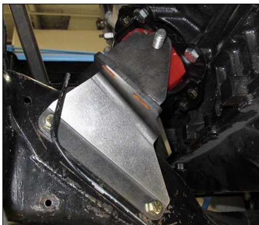
Proper rear-biased left-side supplemental support bracket installation orientation
