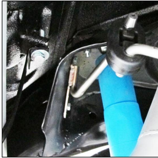
Figure 3 – Rear driver's side hanger (passenger's side hanger is similar)
