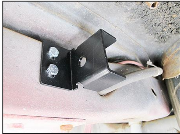
Figure 6 – Right tailpipe hanger bracket orientation
