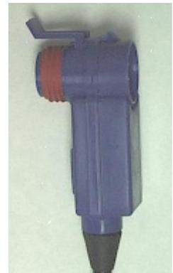
Route and secure the sensor cable from the module and connect the sensor element. If there is excess cable, the cable can be shortened using connector kit P/N 800-CN-TI3P. You should complete the installation and verify operation before shortening the cable.
