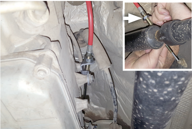
19. Thread nut and locking washer (removed step 16) onto shifter cable then insert cable through bracket.
