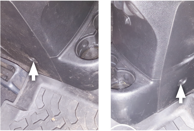
6. Remove screws (x2) securing rear of console. Retain them for later use. Do not remove console from vehicle.
