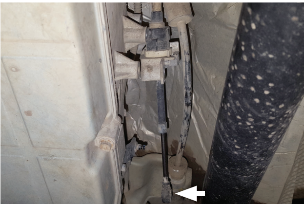
14. Remove shifter cable from transmission as shown.
