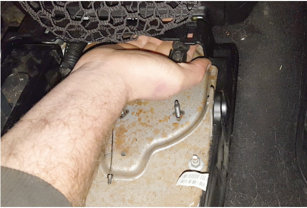
12. Under center controls, push shifter cable and grommet back through hole toward transmission tunnel.
