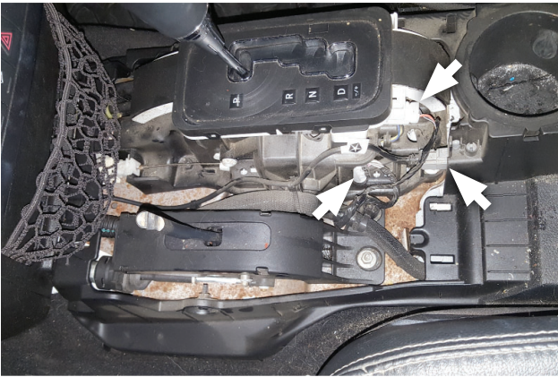
7. Disconnect wiring connectors from shifter and console.
