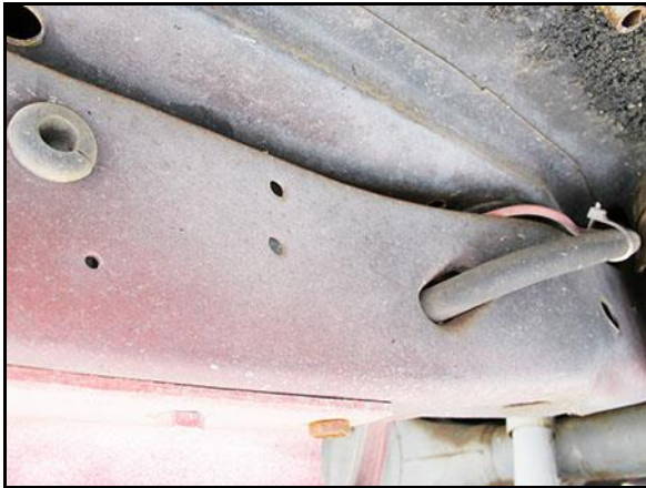
Figure 5 – Right side frame attachment holes
