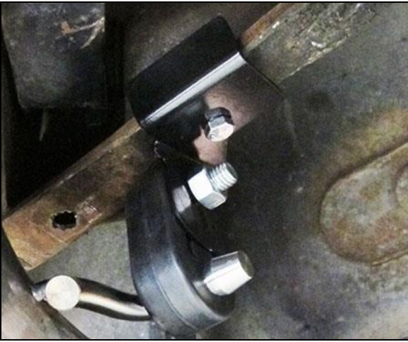
Figure 3 – Left tailpipe hanger bracket
