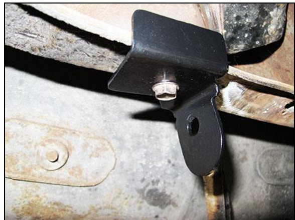
Figure 2 – Right over-axle hanger bracket
