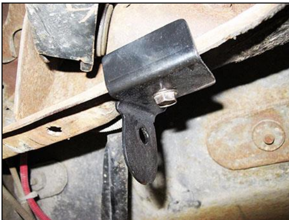
Figure 1 – Left over-axle hanger bracket
