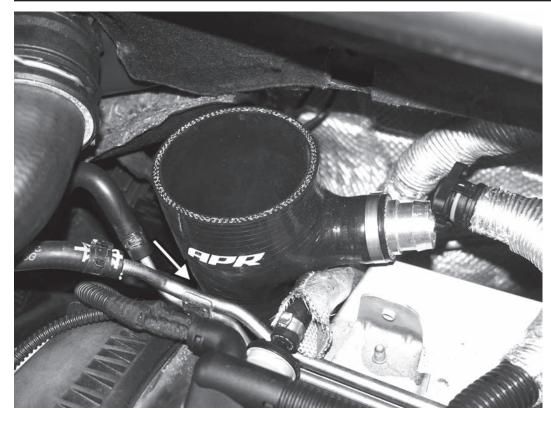
7) Place the APR inlet coupler all the way down onto the turbo inlet. Then rotate the coupler so the PCV hose will easily connect to the port on the side of the APR inlet coupler. Secure the coupler with the spring clamp.
