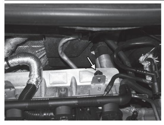
9) Loosely install the previously removed T30 screw into the metal tab on the top of the heatshield.
