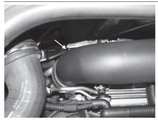
3) Remove the upper spring clamp that holds the rear intake pipe to the top of the coupler at the turbo inlet.
