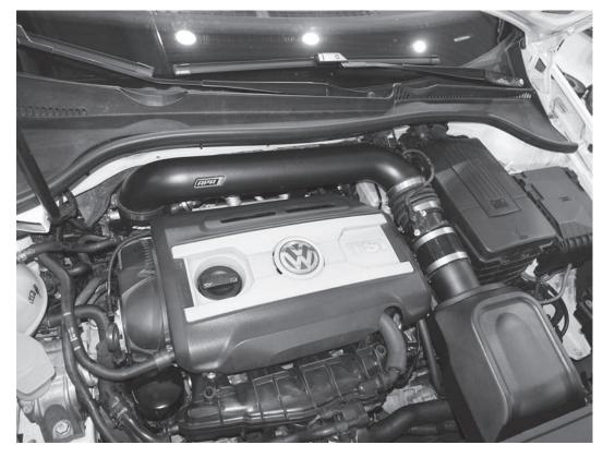
15) Reinstall the engine cover by pushing the four corners down onto the mounting posts on top of the engine.
