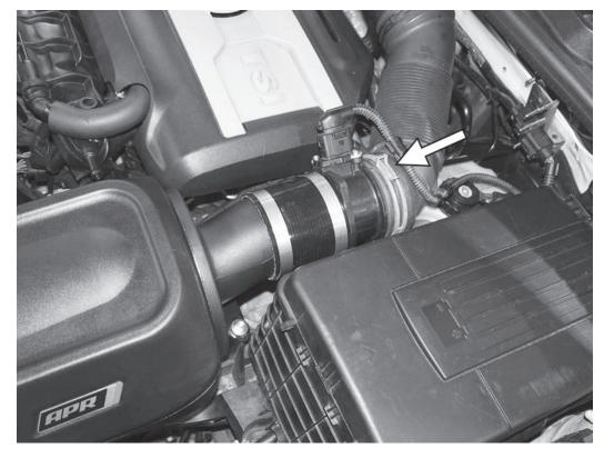
1) Remove the engine cover from the top of the engine by lifting up on the four corners. Using a tool for spring clamps, remove the spring clamp connecting the front side of the accordian inlet pipe to the back of the MAF housing. Separate the accordian hose from the MAF housing.
