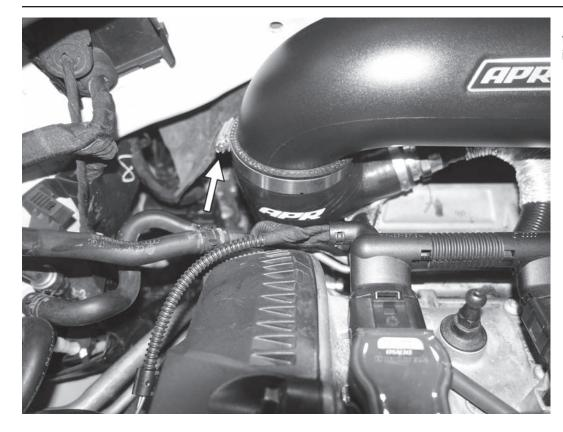
13) Secure the APR intake pipe to the inlet coupler with the previously installed hose clamp.
