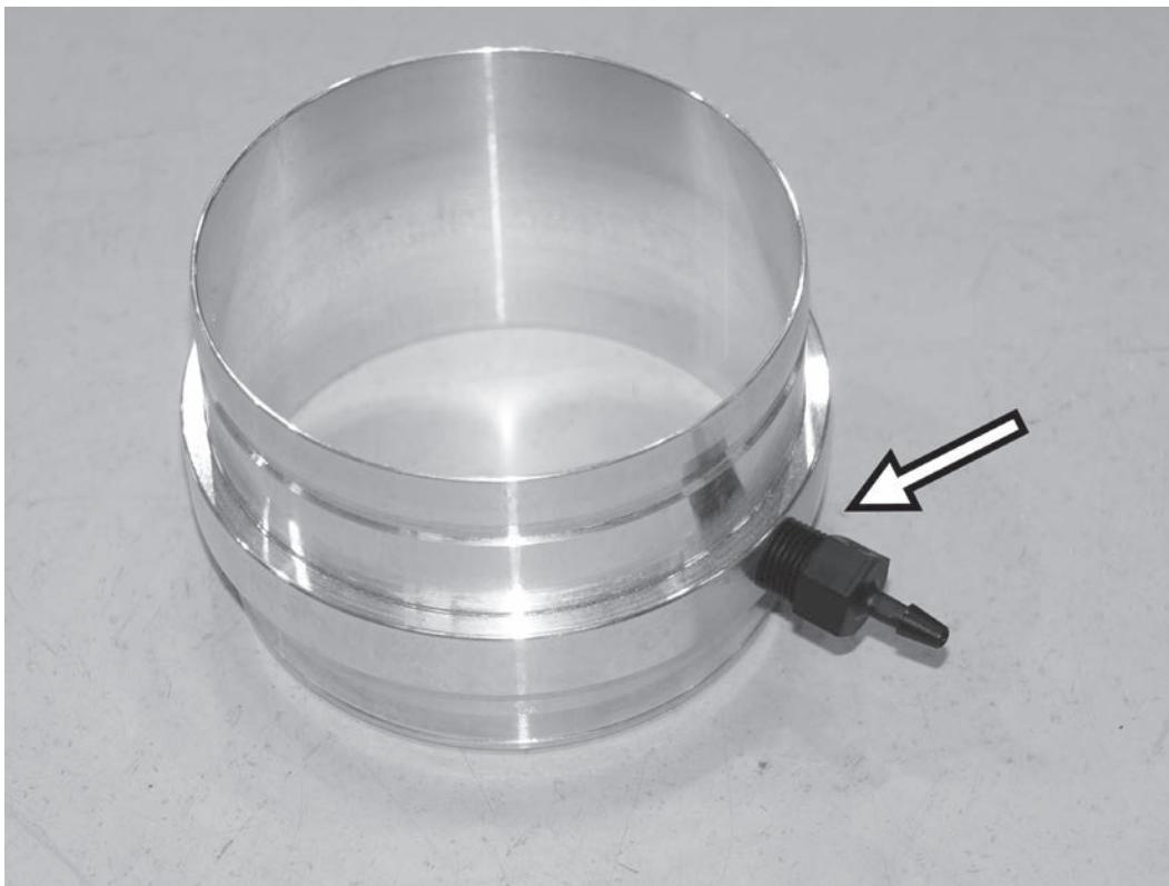
1) Securely screw the vacuum fitting into the side of the APR TSI inlet adapter.
