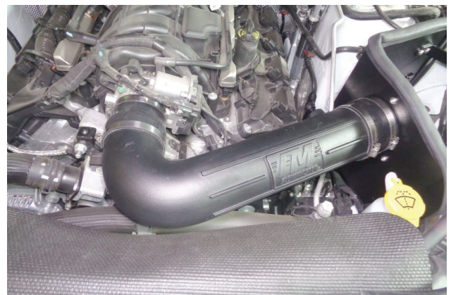
24. Set intake tube into place between heat shield and throttle body as shown without tightening screw clamps.
