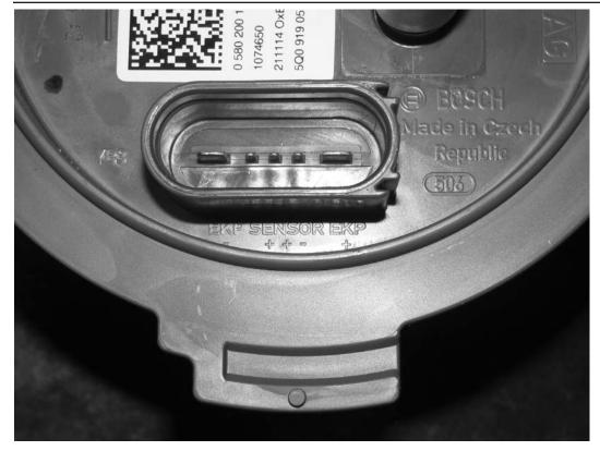
22) Locate and identify the wires inside the pump assembly based off of the markings on the pump top. The AWD pumps have two separate electrical connectors, but the same connections are present.
