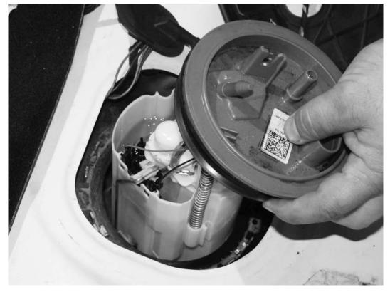
8) Lift up on the fuel pump top, being careful not to damage the rubber seal ring. Remove the seal ring from the car. Be careful not to spill the fuel that is inside the fuel pump basket.
