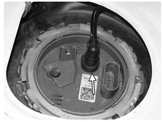
6) Place several rags around the fuel pump area before taking the fuel fitting off. The fuel system may still have pressure in it, so be prepared for spraying fuel. While pressing the tab on the side of the fuel fitting, lift the fitting off the top of the fuel pump. Slide the fitting and hose aside.
