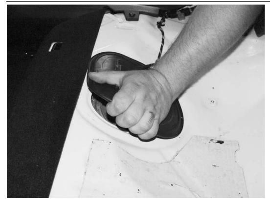
50) Replace the fuel pump access cover, making sure the lip of the cover seals against the metal of the floorpan.
