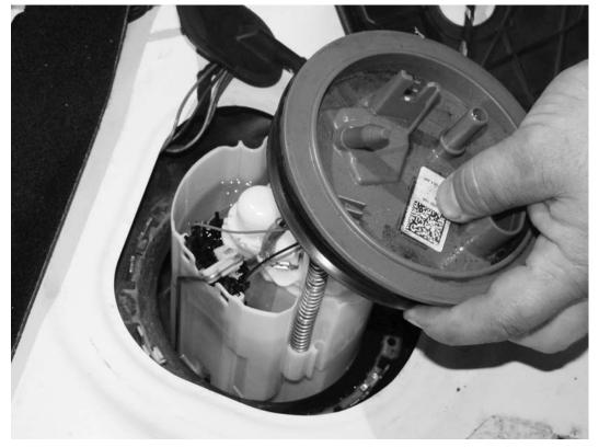
48) Place the factory fuel tank seal around the opening in the fuel tank. Lower the fuel pump assembly slowly into the fuel tank. Finally, carefully push the top of the fuel pump back into the seal being careful not to roll the seal back into the tank.
