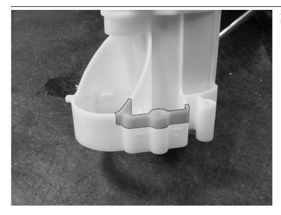
28) Cut 5-6mm off of the side of the pump housing as shown marked.
