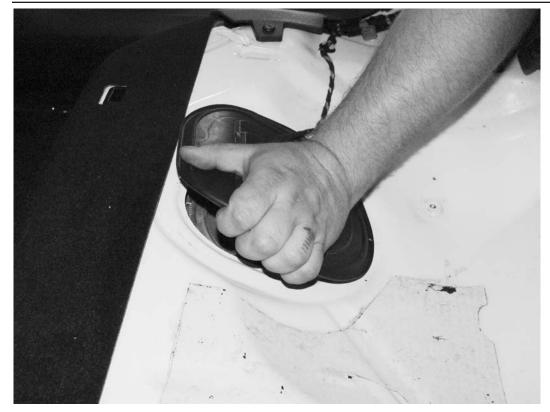
4) Lift up slightly on the fuel pump access cover. Run your fingers all around the cover to separate it from the surrounding metal.
