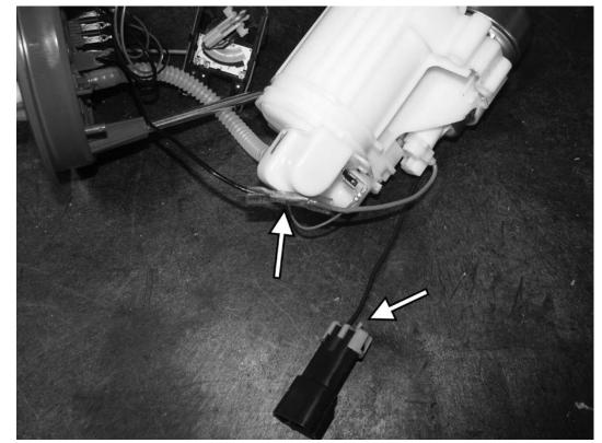
38) Cut the red wire on the APR pump right at the electrical connector attached to the pump. Locate the previously cut, shorter wire that is labeled on the fuel pump top as EKP+. Strip the ends of both wires and connect the red wire from the APR pump with the black wire labeled EKP+ with one of the supplied crimp connectors.
