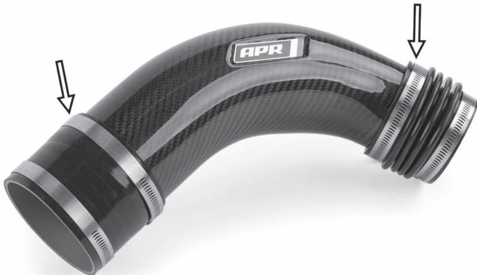
3) Loosely build the shown assembly with the four hose clamps, two couplers, and APR inlet tube. After peeling off the adhesive backing, attach the APR logo in the indented location on the inlet tube.
