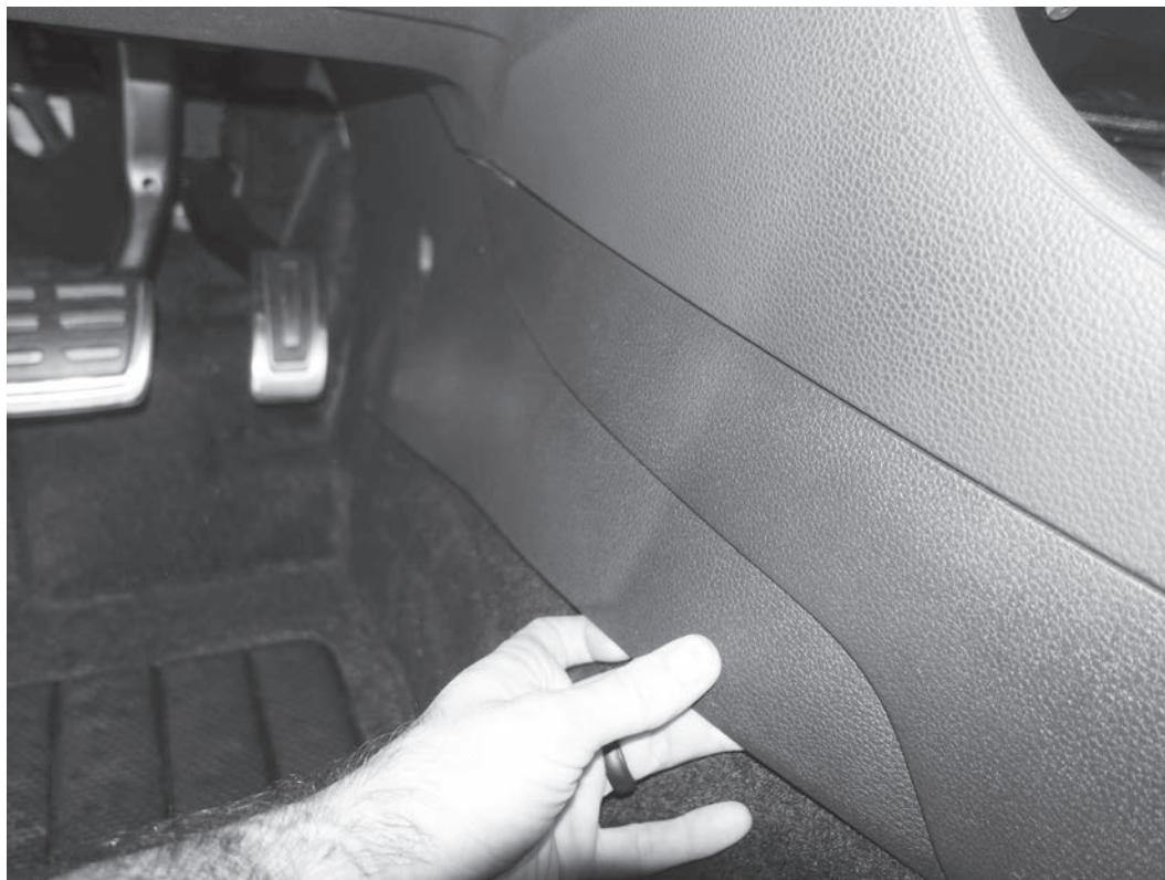
5) Pull the panel down and away to remove it from the car.
