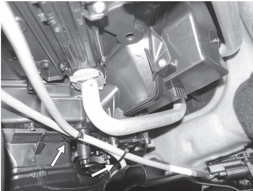
9) Use the remaining cable ties to secure the two cables out of the way.
