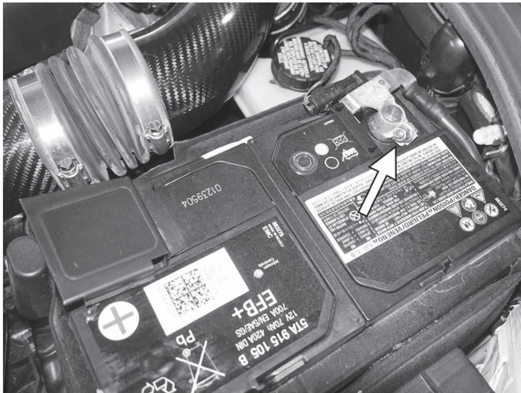
11) Reconnect the negative battery terminal. with a 10MM wrench.
