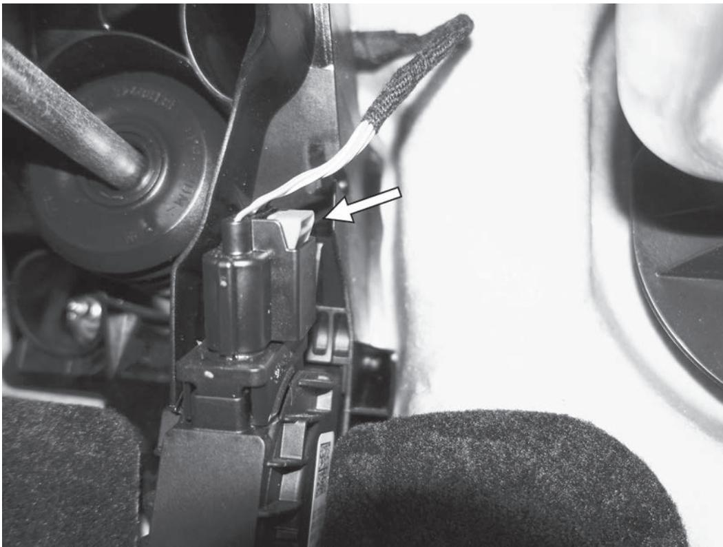
7) On the top of the throttle pedal assembly, disconnect the electrical connector to the throttle pedal. Pull the red tab up and away from the connector before squeezing the red tab to release the connector.
