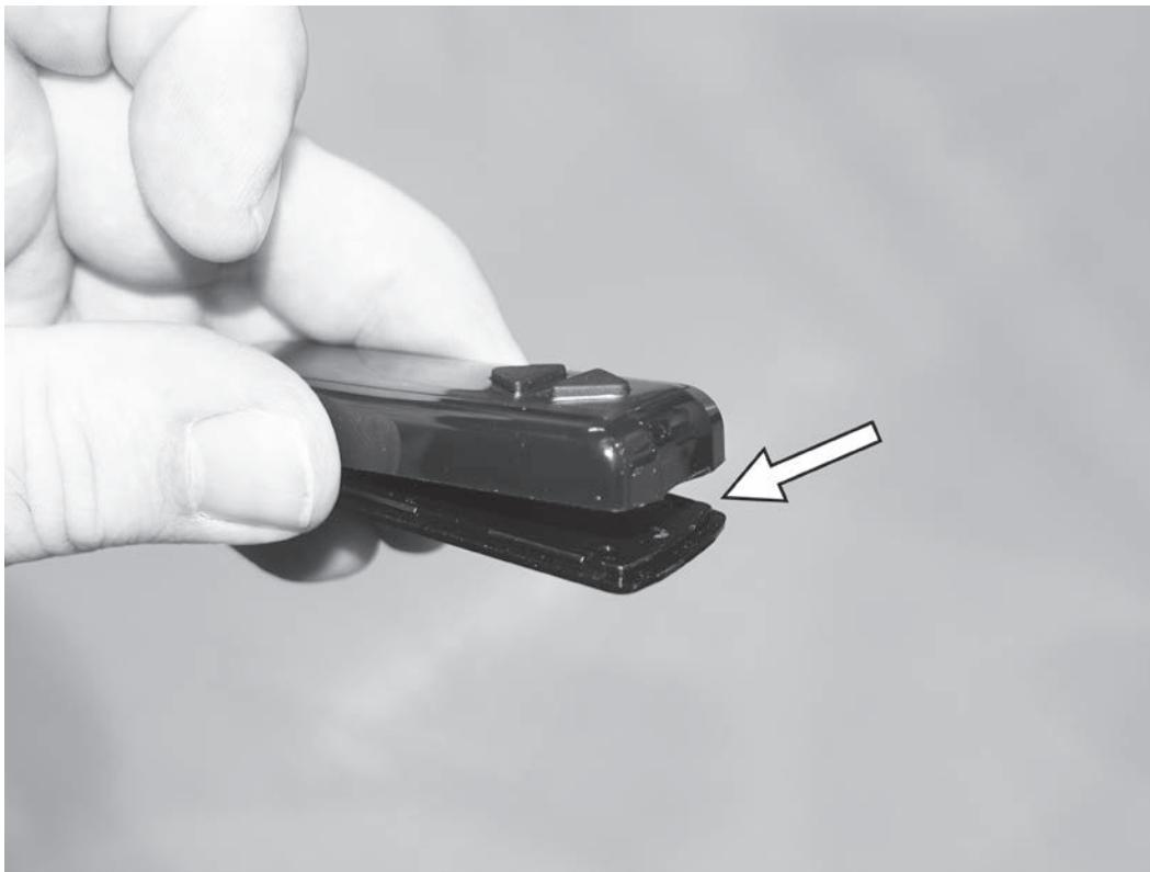
1) Pry open the back of the APR wireless switch. Install the three supplied button batteries.
