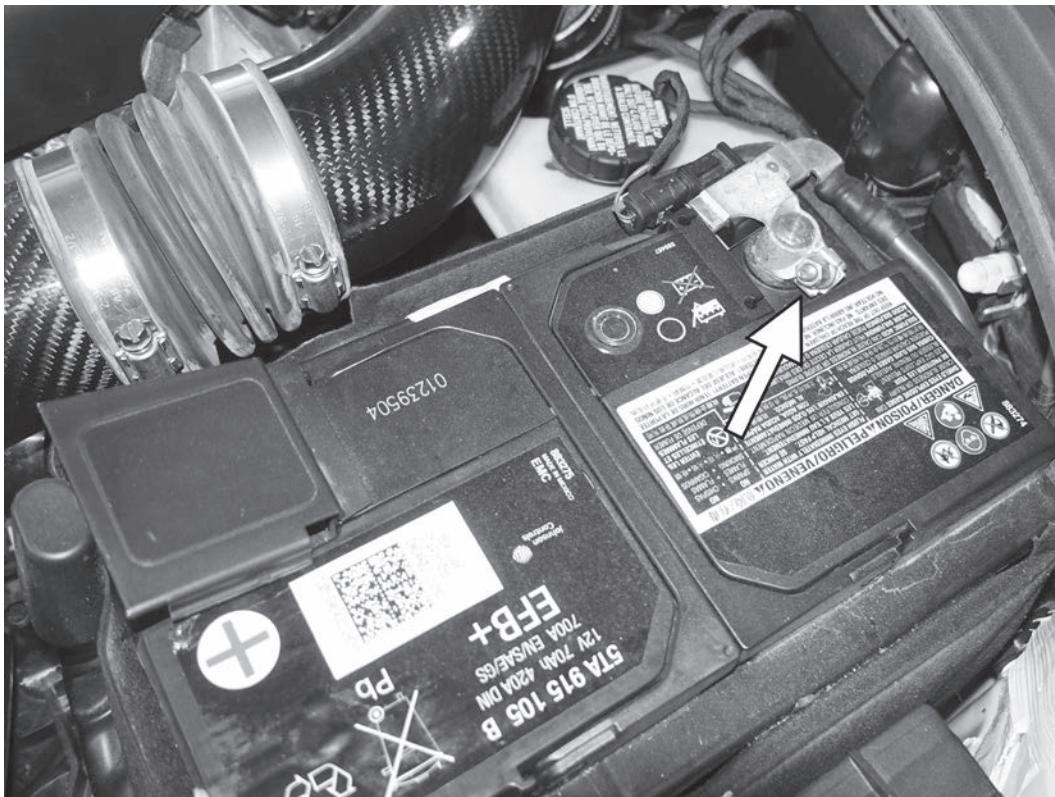
3) Disconnect the negative battery terminal with a 10MM wrench.
