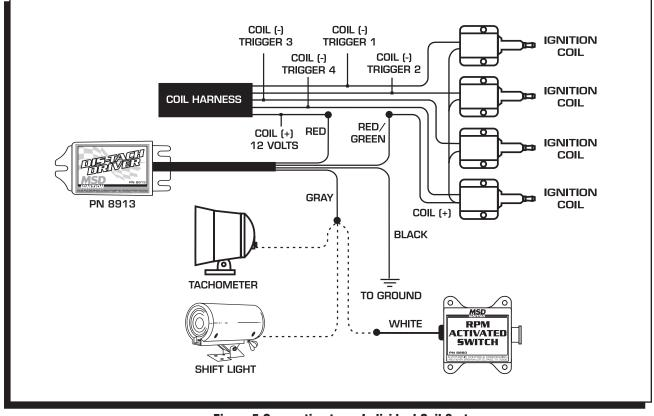
Figure 5 Connecting to an Individual Coil System.
