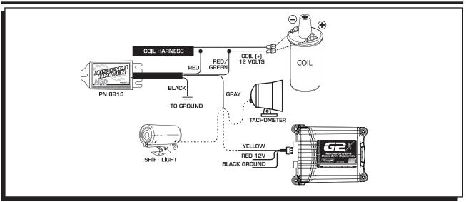
Figure 1 Connecting the MSD G2X with a Points Ignition.
