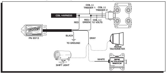
Figure 2 Connecting to a Coil Pack.
