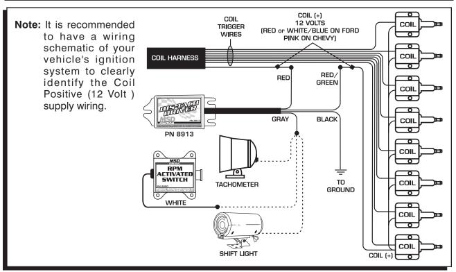
Figure 6 Connecting to Coil Per Cylinder Ford and Chevy.
