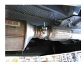
1) Place inlet pipe assembly **#26409S** into position onto the ball connection behind the catalytic converter. Reinstall the clamp onto the ball connection and tighten enough to hold, but still allow for a small amount of adjustment. Connect the hanger on the pipe to the rubber mount on the vehicle.
