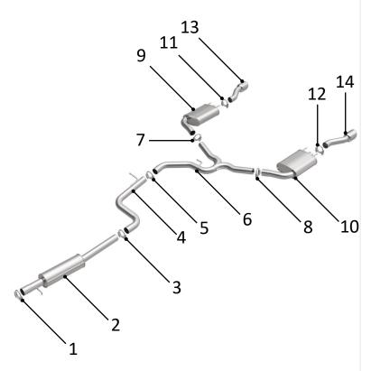
**STEP 1:** (Carefully read all instructions before installation) Disconnect the vehicle's battery before removal of the OEM exhaust system. This will prevent electrical accidents and will reset the computer if it applies to the vehicle. Remove existing exhaust system from the vehicle. Only remove parts that will be replaced. Clean existing flange with a wire brush to ensure proper sealing.
