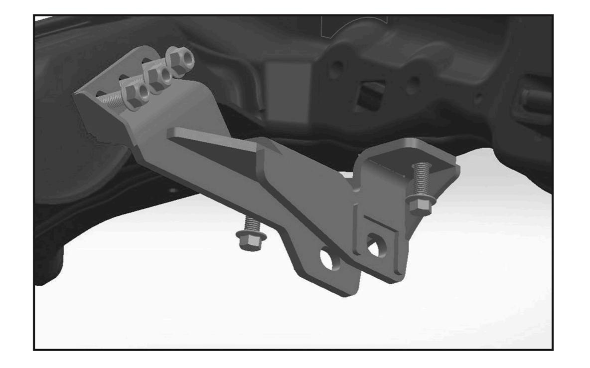
Install cams with bolt hole towards passenger side
