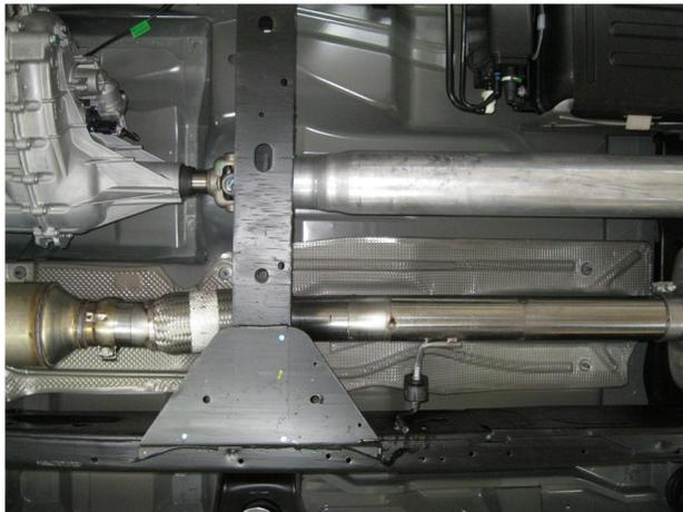
**Step 2.** To begin, fasten the Inlet pipe assembly to the catalytic converter using the OEM clamp assembly and by fitting the welded hanger into the OEM rubber insulator (Leave all clamps and fasteners loose for final adjustment of the complete system.)
