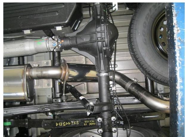
**Step 3.** Install the Muffler to the Inlet Pipe Assembly using the supplied 3.50" clamp. Next install the over axle Resonator assembly to the Muffler in the similar fashion using the supplied 3.50" clamp, fitting the welded hangers into the rubber insulators.
