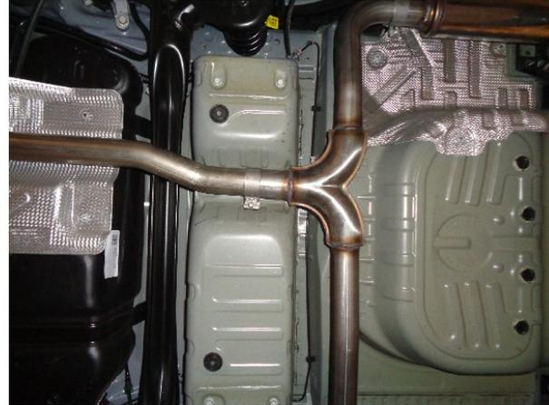
**Step 3:** Next loosely fasten the Y-Pipe Assembly to the Resonator Assembly using the supplied 2.25" clamp.
