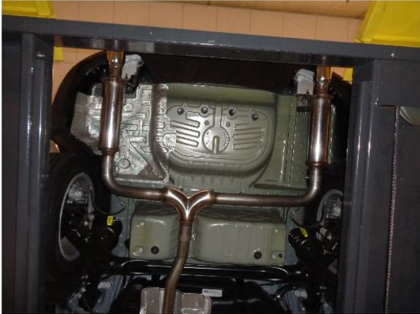
**Step 5:** Next slip the P/S Muffler Assembly onto the Y-Pipe Assembly and loosely fasten with the supplied 2.25" Clamp. Using the supplied Rubber insulators attach the hangers. Fit the D/S Muffler Assembly in the same manner using the supplied clamp and OE rubber insulators.
