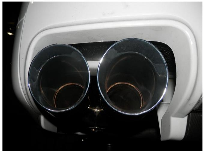
**Step 4.** Loosely install both Tail Pipe Assemblies using the supplied clamps.
