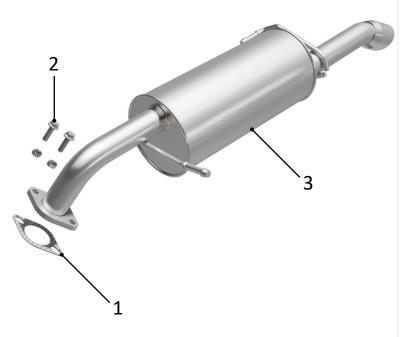
(Carefully read all instructions before installation) Disconnect the vehicle's battery before removal of the OEM exhaust system. This will prevent electrical accidents and will reset the computer if it applies to the vehicle. Remove existing exhaust system from the vehicle. Only remove parts that will be replaced. Clean existing flange with a wire brush to ensure proper sealing.
