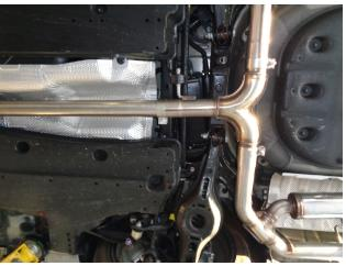
Step 2. Begin installation of the MagnaFlow system by attaching the Inlet Pipe Assembly to the outlet of the catalytic converter using the OE fasteners. Next, attach the Y-Pipe Assembly using the supplied 2.50" clamp and engaging the hanger into the rubber insulators. (Leave all clamp and fasteners loose for final adjustment of the complete system.)
