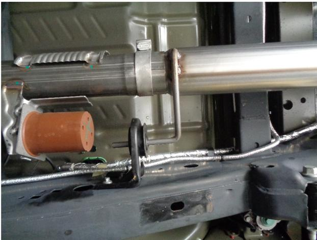
**Step 2.** Install Inlet Pipe Assembly. Loosely fasten it to the DPF outlet using supplied clamp.
