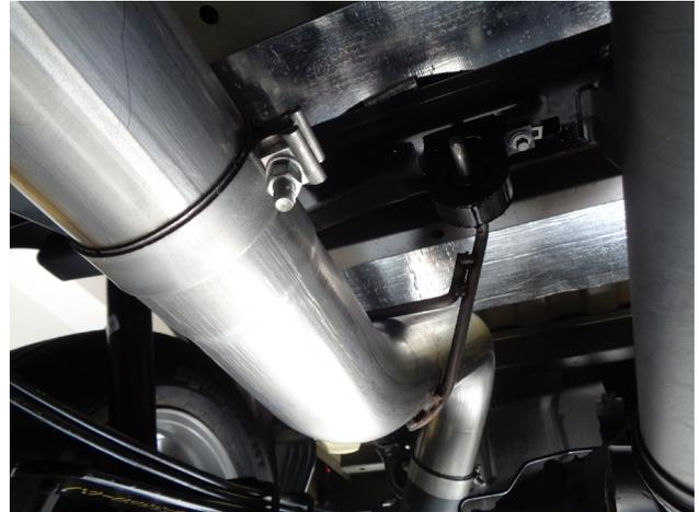
**Step 3.** As you assemble the Extension Pipes loosely locate the Hanger Clamp Assemblies as needed then install the over axle pipe.
