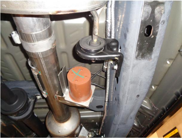
**Step 1.** Working front to rear loosen or remove all OEM band clamps and disengage all welded hangers from the rubber insulators. Be sure to retain all mounting hardware as it will be needed to install your new MAGNAFLOW system. Slide the OEM system off towards the front of the vehicle.
