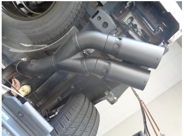
**Step 4.** Install the Tail Pipe Assembly in the same way. Once a final position has been chosen for the new exhaust system, evenly tighten all clamps from front to rear using the torque specifications on page one of the instructions. Inspect all fasteners after 25-50 miles of operation and re-tighten if necessary.
