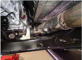
**Step 1.** To remove the OEM exhaust system disengage the welded hangers from the rubber insulators and remove the tailpipe assy. Unfasten the clamp attaching the OEM inlet pipe assembly to the catalytic converter. Do not damage or discard the inlet pipe clamp or rubber insulators as they will be re-used to mount the new system. Disengage the inlet pipe assembly hanger and remove the exhaust from the vehicle.
