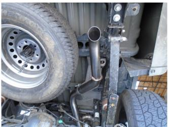
**Step 5.** Loosely install the Over Axle Pipe and Tail Pipe Assemblies locating the welded hangers to the rubber insulators and secure using the supplied clamps.
