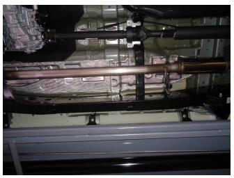
**Step 2.** To begin, loosely fasten the Inlet pipe assembly to the outlet of the OE catalytic converter using the Supplied clamp. Engage the welded hanger into the rubber insulator (Leave all clamps and fasteners loose for final adjustment of the complete system.)
