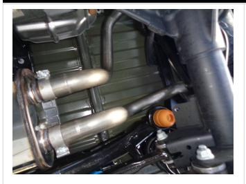
Step 5: Next, attach the driver side and passenger side mid pipes to the mufflere and loosely tighten.
