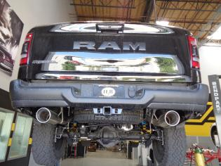
Step 7: Using the supplied rubber insulators install the tailpipe assemblies to the mid pipes fitting the hangers into the installed hanger brackets.
