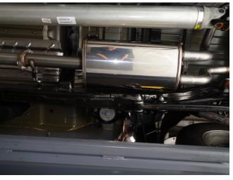
Step 3: Install the new system by attaching the muffler assembly to the resonator pipe assembly with supplied hardware and gasket.
