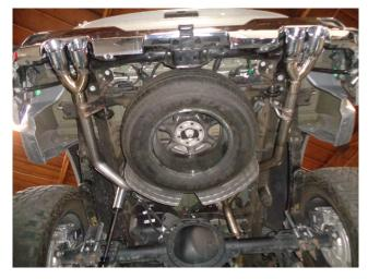
Step 5. Complete the installation by attaching both Tailpipe Assemblies to the Y-Pipe Assembly using the Supplied 2.50" clamps.
