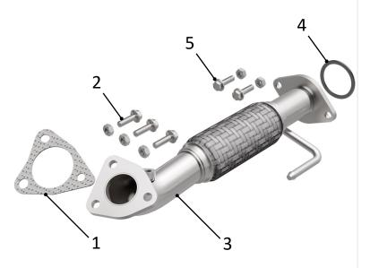
(Carefully read all instructions before installation) Disconnect the vehicle's battery before removal of the OEM exhaust system. This will prevent electrical accidents and will reset the computer if it applies to the vehicle. Remove existing front pipe from the vehicle. Only remove parts that will be replaced. Clean existing flange with a wire brush to ensure proper sealing.
