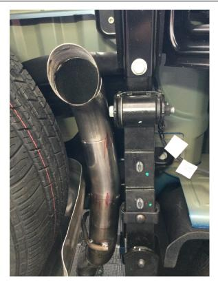
**Step 7:** Finish by Installing the Tail Pipe to the Over Axle Pipe outlet using the supplied clamp. Engage the hanger to the OE rubber insulator. Clearances are very tight, make sure there is adequate room after tightening.
