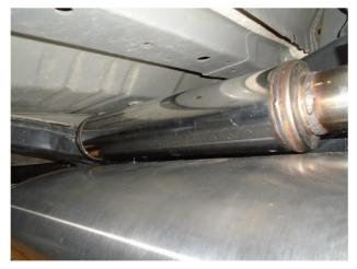
**Step 5:** When using the NDT chamber, mount it above the muffler as shown. Be sure to leave at least 1/2" of clearance between both components.
