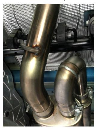
**Step 6:** Install the Over Axle Pipe to the Muffler outlet using the supplied clamp. Engage both hangers to the OE rubber insulators.
