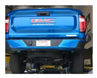
**Step 8:** Once a final position has been chosen for the new exhaust system, evenly tighten all clamps from front to rear using the torque specifications on page one of the instructions. Inspect all fasteners after 25-50 miles of operation and re-tighten if necessary.
