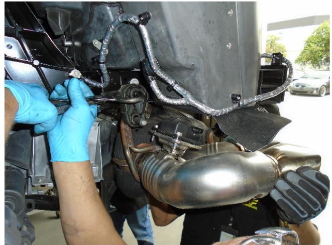
Step 16. Support the OEM exhaust system as you disengage the drivers and passengers side hanger rubbers. The OEM system can now be removed. With the OEM system removed unbolt the valve motors from each valve. Retain all mounting hardware as it will be needed to install your new MAGNAFLOW system.
