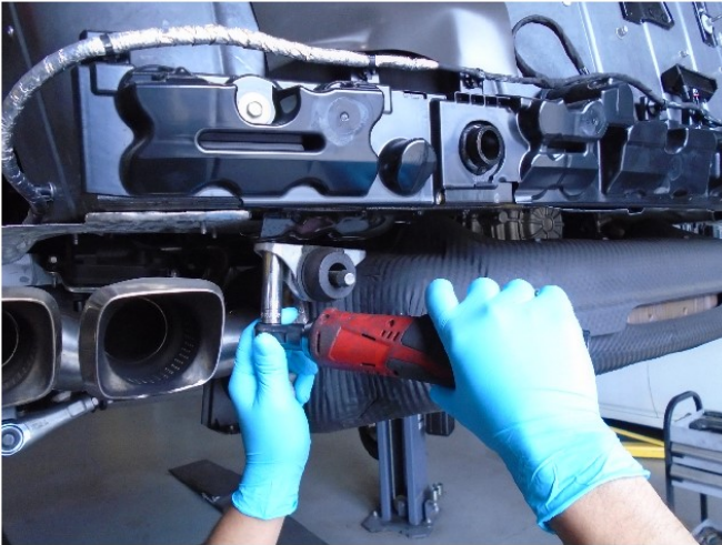
Step 13. Remove the (4) 13mm bolts attaching the two rear hanger brackets.
