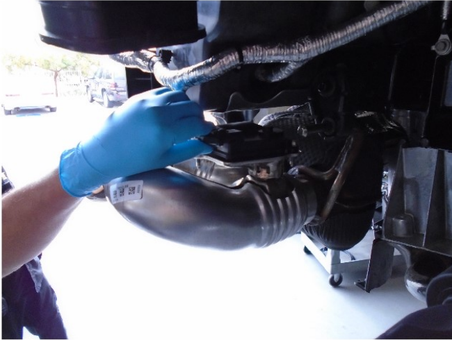
Step 12. Unplug both of the rear valve motors.
