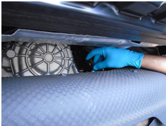
Step 14. Once the hanger brackets have been removed the exhaust system will drop enough to allow access to the front valve motors. Disconnect both valve motors.
