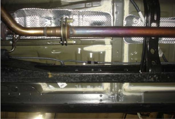
**Step 1.** Begin removal of the OEM exhaust system by unbolting the two spring loaded bolts attaching the exhaust to the catalytic converter. Do not discard or damage the OEM fasteners or rubber insulators as they will be used to install the new system.
