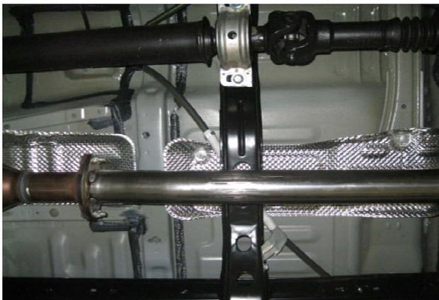
**Step 3.** Begin installation of your new MAGNAFLOW system by attaching the Inlet Pipe Assembly to the catalytic converter outlet using the OEM fasteners and insulator. Keep all fasteners and clamps loose until final adjustment.
