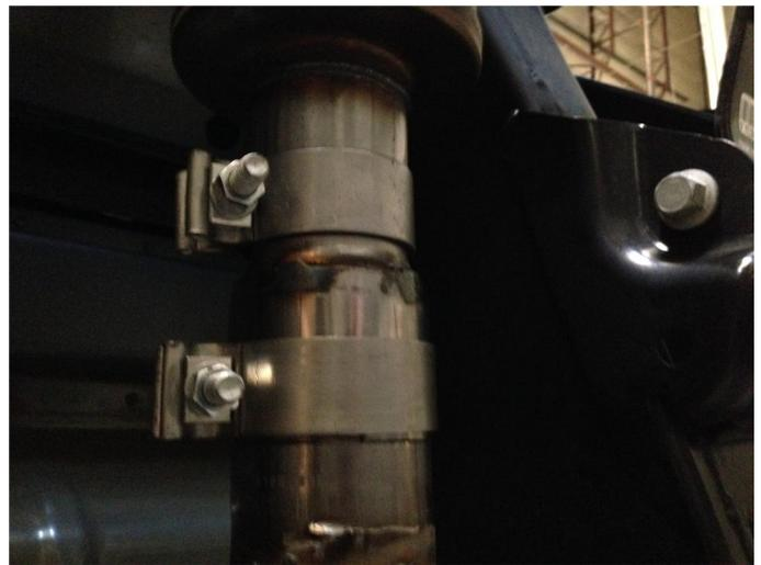
**Step 3.** Install the Extension Pipe between the Inlet Pipe Assembly and the Muffler Assembly using the supplied 3.00" and 2.50" clamps. Engage the welded hanger to the rubber insulator.
