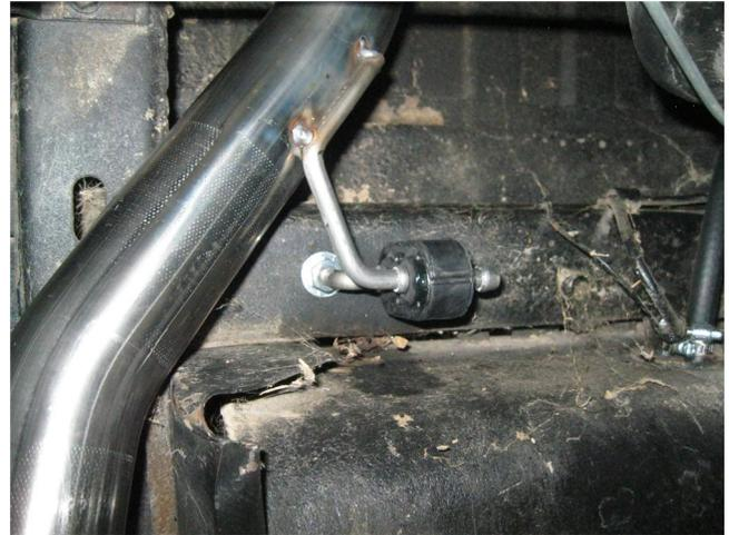
**Step 3.** Before installing the Tail Pipe Assemblies you will need to install the supplied threaded hangers into holes in the frame rails behind the rear differential using two supplied nuts and washers to adjust height and lock into place.
