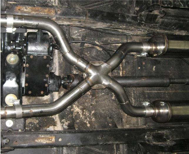
**Step 1.** After removal of the OEM system you can begin installation of the Magnaflow system. Start by attaching the X-Pipe Assembly to the factory outlets using the supplied 2.5" clamps. Leave all clamps and fasteners loose until final adjustment.
