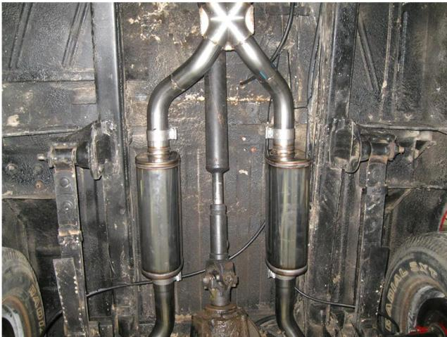
**Step 2.** Next install the mufflers as shown (be aware of orientation) using the supplied 2.5" clamps.
