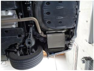
Step 1. To remove the OE exhaust system begin by unfastening the 2 bolt flanges, one located at the front of the vehicle (behind the catalytic converter assy) and one at the rear (by the muffler). Working front to rear disengage the hangers from the rubber insulators and remove the exhaust. Do not damage the rubber insulators and retain front flange hardware as they will be used to install the new exhaust system.
