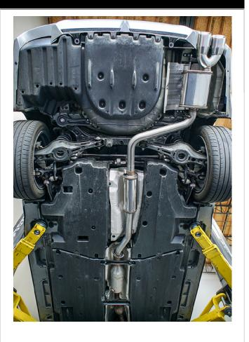
Step 2. Begin installation of the MagnaFlow system by attaching the Resonator Assembly to the outlet of the catalytic converter using the OE fasteners. Next, attach the Muffler Assembly using the supplied 2.50" clamp and engaging the hangers into the rubber insulators. (Leave all clamp and fasteners loose for final adjustment of the complete system.)
