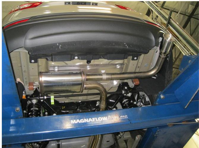
**Step 5.** Install the Mid Pipe, Muffler Assembly and Tail Pipe Assembly using a similar method. Locate the welded hangers to the OEM rubber insulators.
