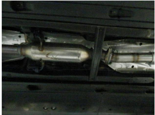
**Step 2.** This Magnaflow exhaust system will fit both a 2.0L Turbo and a NA 2.4L Optima depending on which Inlet pipe Assembly is used (both are supplied). The 2.0L Turbo Inlet Pipe has the slotted flange. Begin installation of the new system by fastening the correct Inlet Assembly to the resonator outlet using the OEM fasteners (Leave all clamps and fasteners loose for final adjustment of the complete system.)
