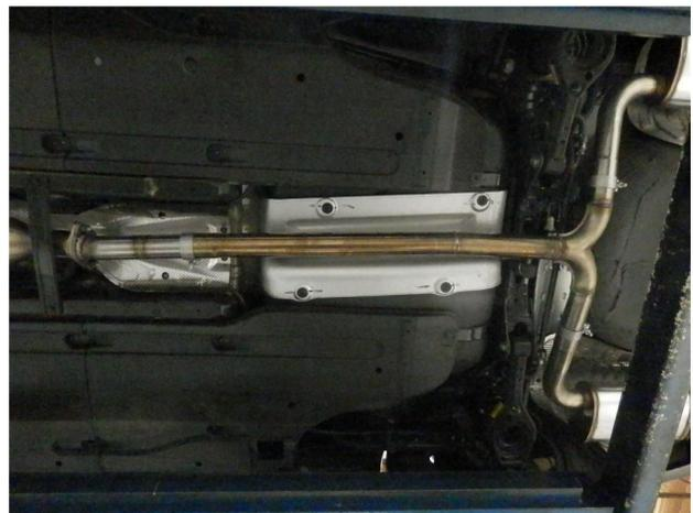
**Step 3.** Next Install the Y-Pipe Assembly to the Inlet Pipe Assembly using the supplied 2.50" clamp. Insert hanger into rubber insulator.
