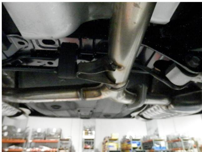
**Step 1.** To extract the OEM exhaust system begin by un-fastening the flange located behind the resonator and the second flange located in front of the Driver side muffler assembly. Next, working rearward, disengage all welded hangers from the rubber insulators. Do not damage or discard the rubber insulators or fasteners as they will be re-used to mount the new system. You can now remove the exhaust from the vehicle.
